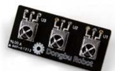
X1 DRI-0013 IR Receiver PCB
